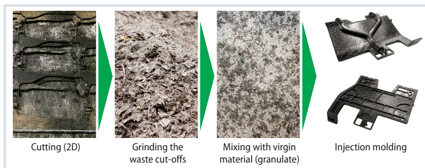
Fig. 3. Tepex organosheets are easily recycled and subsequently reused for technical components. Strength, stiffness, and toughness of the recyclate correspond to those of short fiber-reinforced plastics with the same fiber contents Source: Lanxess; graphic: © Hanser
